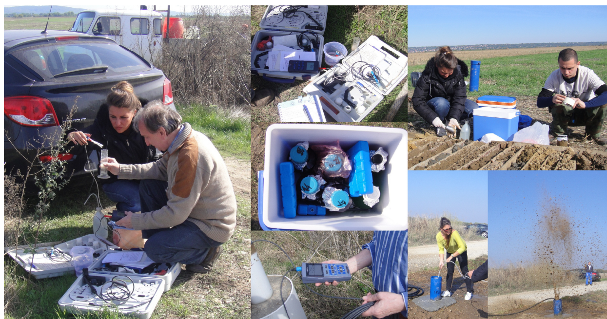
Figure 6. Groundwater and soil sampling during the construction of piezometer Pb-12', in situ measurement and piezometer rinsing (photo Jelena Zarić - September 2013)
